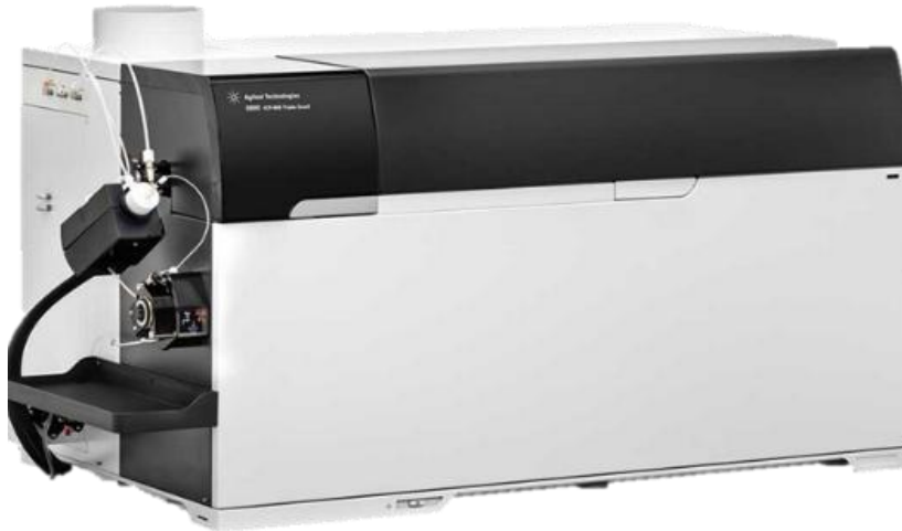
Figure 36 QQQ ICP-MS (Agilent 8900) used to analyse trace element compositions in Li-bearing samples in the MADITRACE project.
