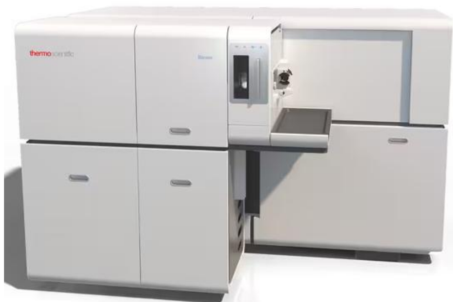
Figure 8 Neoma™ MS/MS MC-ICP-MS instrument for S isotopic analysis. (Image source: Thermo Scientific™ website)
