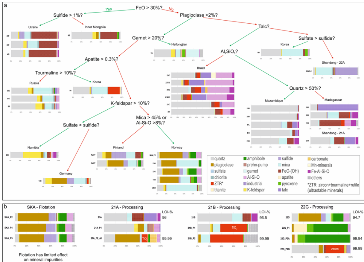
Figure 28 a) A possible decision tree to distinguish between traded graphite concentrates based on their mineral impurities ( \delta > 2.46 \text{ g/cm}^3 ). All values are in area%. b) Traceability of the mineralogical signature along the value chain.
