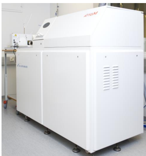
Figure 3 Nu AttoM single-collector ICP-MS used for trace element analyses at GTK.
